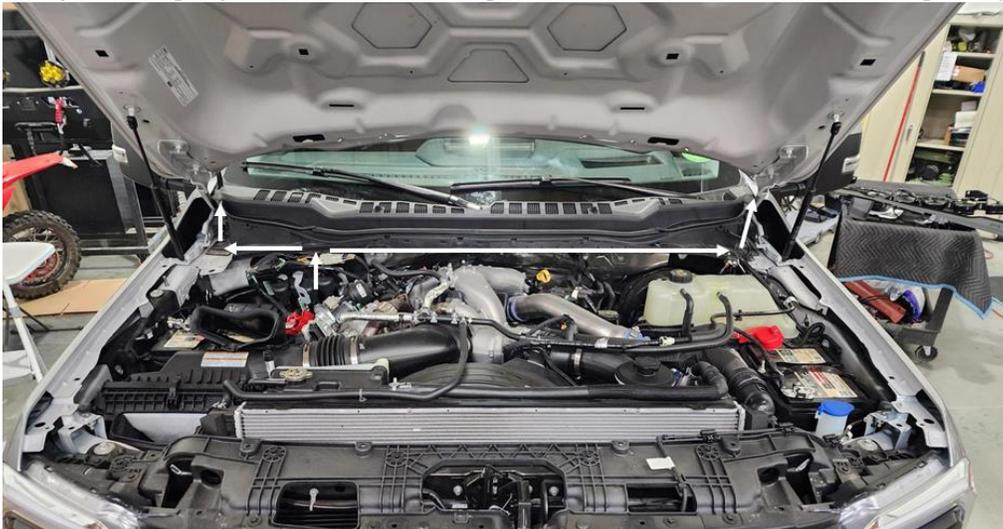
With the 10mm socket, attach the red ring terminal to the positive post of the battery.
