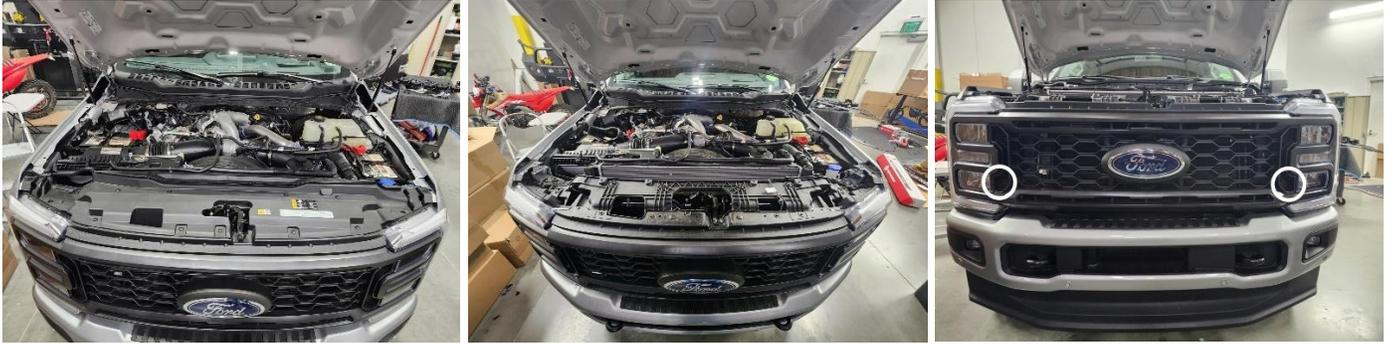
2. Carefully pull the front grill out disengaging the plastic clips. Remove the electrical connector and water line from the grill to free it. To remove the water line, remove the small black plastic ring and pull.
