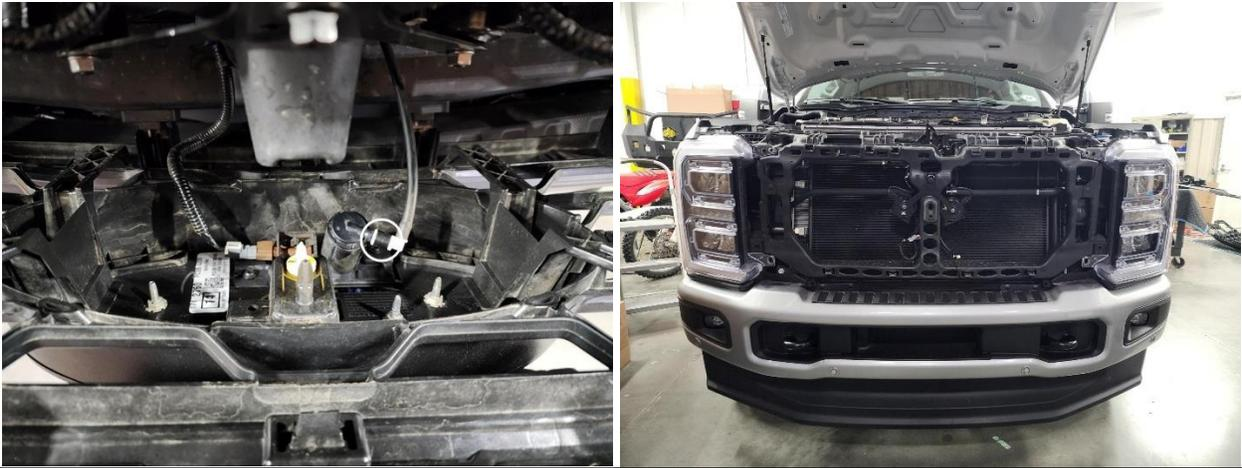
Remove the 2x 10mm bolts from the top of the DS headlight and the 13mm from the bottom by accessing it from the fender well. Pull the headlight out and remove the electrical connectors on the back. Find the included backlight wiring harness and locate the scotchlok connector. For trucks with stock LED headlights, place the scotchlok connector around the wire coming from Pin 8. For trucks with halogen bulbs, place the scotchlok around the Pin 2 wire of the two-pin connector.
