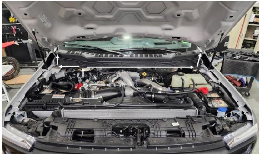
Carefully cut back the sheathing on the upfitter harness around the wiring till the black wire can reach the negative battery terminal without straining. Attach the black wire to the negative battery cable and reattach the cable to the battery.
