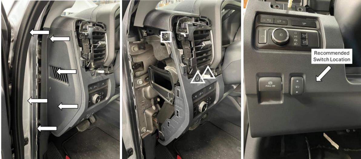
Take a reference photo of the switch's wiring output. Disconnect the spade connectors and run the wires through the newly created switch hole. Reconnect the wires and press the switch into place.
