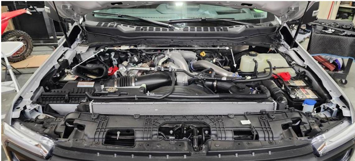
Locate the white connector that attaches the switch to the main harness and disconnect it. With a pick, remove the wire terminals from the connector. Run the wires switch lead, terminals first, through the wire passthrough (circled) starting inside the cab. Reinstall the terminals into the connector and reattach it to the main harness.
