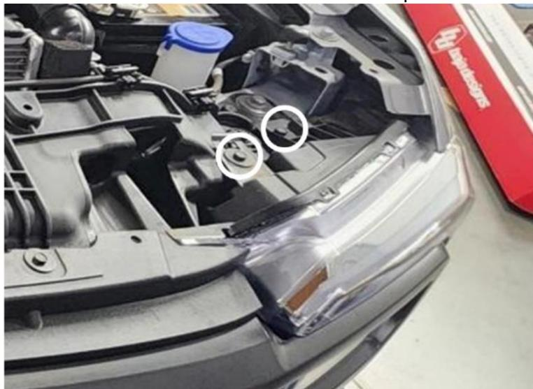
4. Route the wire lead to the LP4s. Using a flathead screwdriver, remove the green cover on the front of the Deutsch connector of the main harness. Insert the wire into the #3 position until it clicks into place and replace the cover. Repeat for the other light. Tie all excess wire into a service loop and reinstall all removed components.
